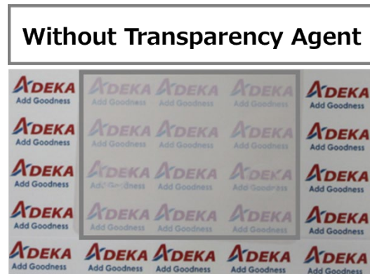
Polypropylene test piece (1 mm) without the addition of a clarifier
