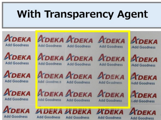
Test piece (1 mm) made of polypropylene with 0.1% TRANSPAREX
