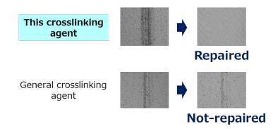
※ A comparison after heating at 120℃ for 24hours. Glass was coated with plastic containing 10% of crosslinking agents and was scratched by pencil.
