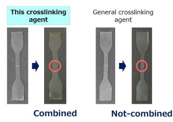
※ A comparison after heating at 120℃ for 24hours. A plastic containing 10% of crosslinking agents and was cut by knife.
