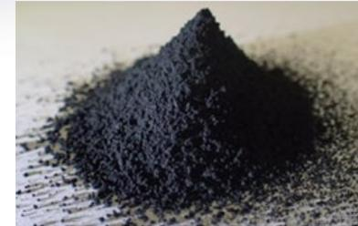
Electrode active material for next-gen. rechargeable batteries **SPAN**
