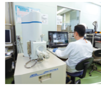
Exterior observation and determination of constituent elements using an analyzer
