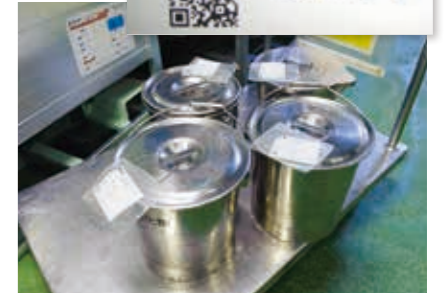
Management through QR code Labels with QR codes are pasted onto all raw materials. All processes, from the receipt of raw materials to production and shipping, are managed through the traceability system using the QR codes.
