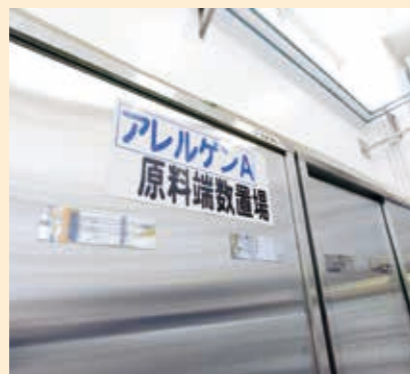
Switching from stickers to stainless steel plates
